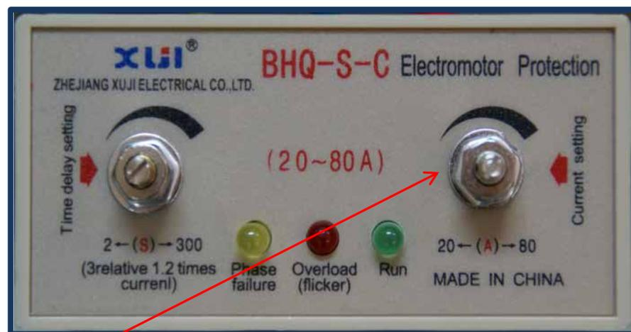
2. Adjust the “current setting screw” to the maximum on the electronic protector (BHQ-S-C) by turning it clockwise.
