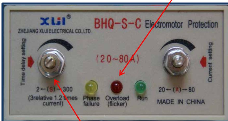
6. In order to set the “time delay setting” on the above mentioned unit, refer to the Amp meter on the front of the unit and set the delay for a bit longer than the starting time of the motor. The centre of the set screw should be around 150 seconds.
