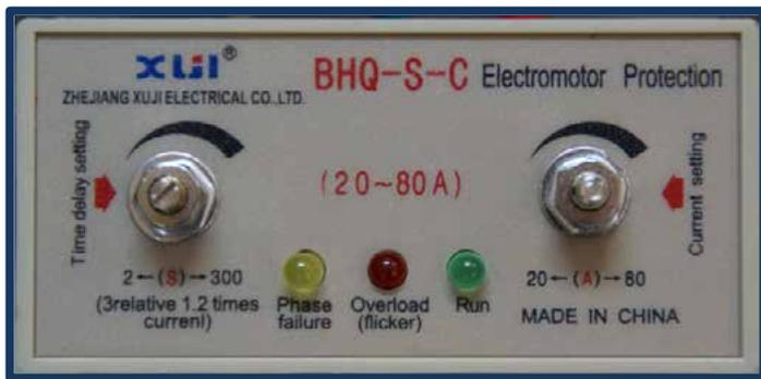
In the event of phase loss or an overload condition, the green and red LED lights on the electro motor protection (BHQ-S-C), inside the main unit, will light up and indicate the relevant condition.
